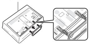
4 Insert and tighten the M5 screws (length: 14 mm) into the holes on the rear of the TV.
